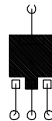
b. 95^\circ\text{C/W} when mounted on a 0.066\text{ in}^2 pad of 2oz Cu.
